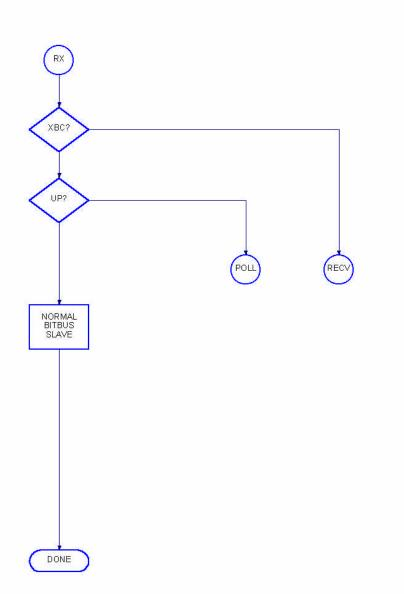
If an XBC is received by a slave, it will check the layer 2 PDU's ADR field first. If it is NOT equal to the own node address, it is a simple broadcast and the layer 2 will pass the message to the user (layer 7) without any further action.
