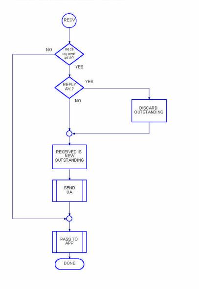
If a slave is polled using the UP command, it checks, if there is an outstanding XBC. If there is no, the slave will not take any action. If there is one, the slave checks whether the user (layer7) has already handled the XBC and if it is ready send. In this case the slave sends the XBC reply otherwise it sends an UP itself.
